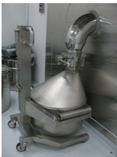
Stopper discharge from autoclave
